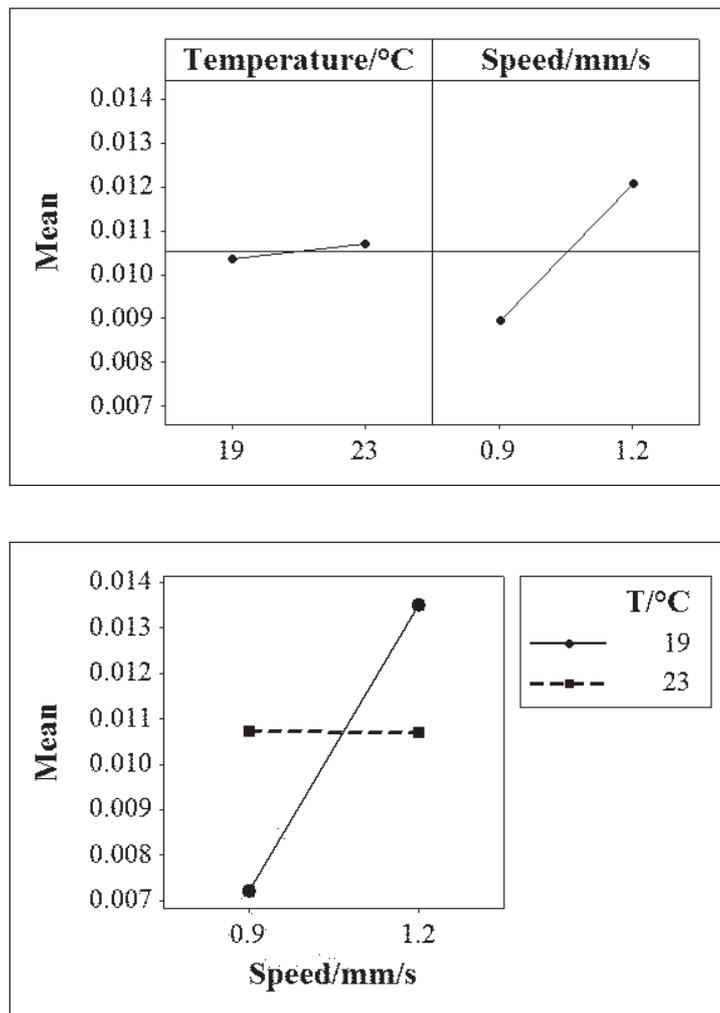
Figure 7: Main effects of quantitative factors (temperature and speed) on measurement variability (a), and relevant interaction (b).
