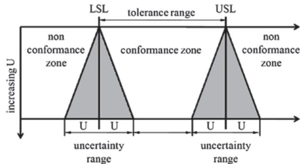
Figure 1: Effect of measurement uncertainty on conformance zone (Lanza *et al.*, 2010)
