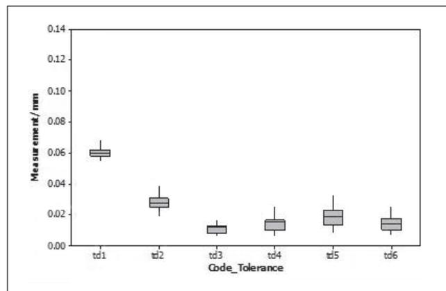
Figure 6: Boxplot of results obtained for tolerated features in qualified probe condition.
