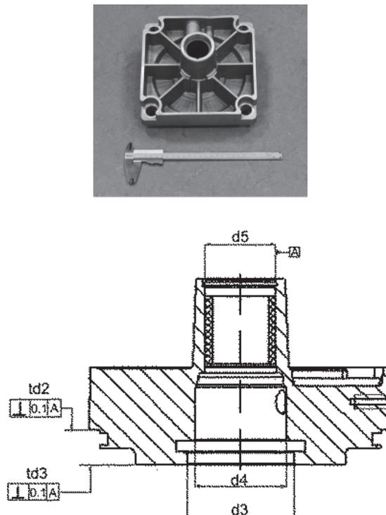
**Figure 3: Measured workpiece (a), and cross section showing main dimensions and features with tolerances  $td2$  and  $td3$  considered (b);**
