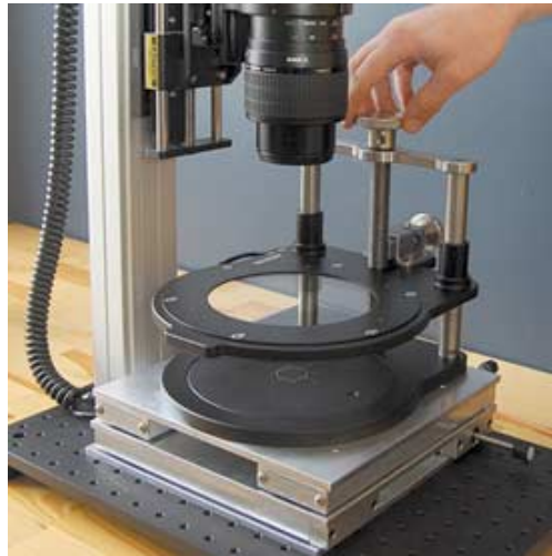
Figure 5: Gel-Sight equipment will photograph an object six times each with light from a different angle. Computer-based systems will incorporate the six photographs together for a 3D image.
