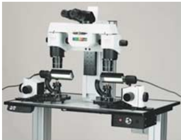
Figure 1: The comparison microscope is the primary tool of an examiner. Examiners can view two objects at the same time through the optical bridge under magnification.
