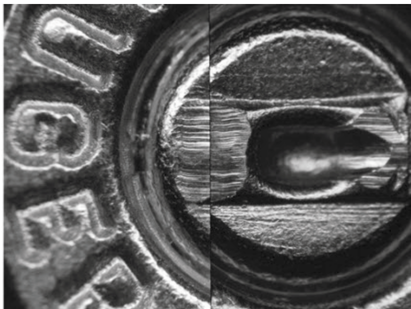
Figure 3 depicts the side-by-side comparison of two test-fired cartridge cases from consecutively manufactured (different) firearms. In contrast to Figure 2, the marks from each cartridge demonstrate a lack of significant correspondence.
